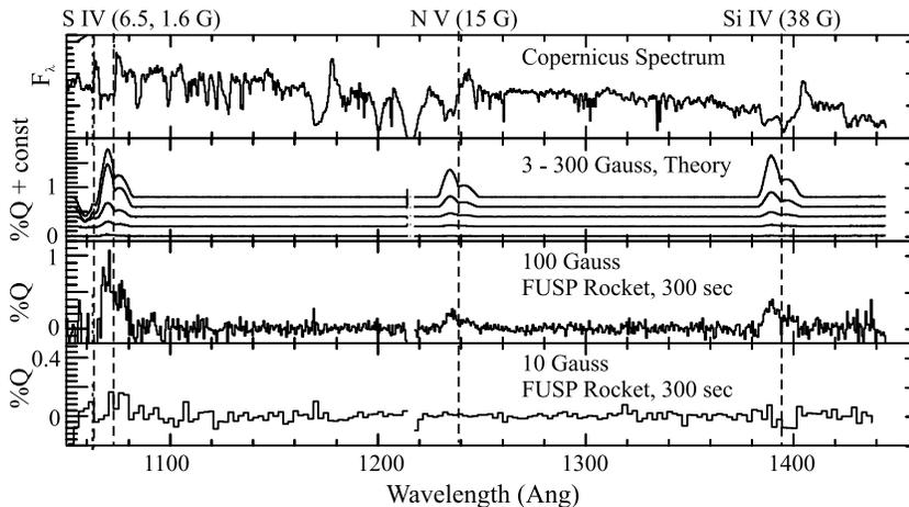
Figure 1. A simulated FUSP observation of  $\zeta$  Ori. Top: Copernicus spectrum. Second panel: theoretical polarization profiles for three resonance lines,  $B_{Han}$  listed at top. Bottom panels: simulated 300 sec FUSP observations for base wind fields of 100 Gauss (unbinned) and 10 Gauss (binned to  $2.4\text{\AA}$ )
