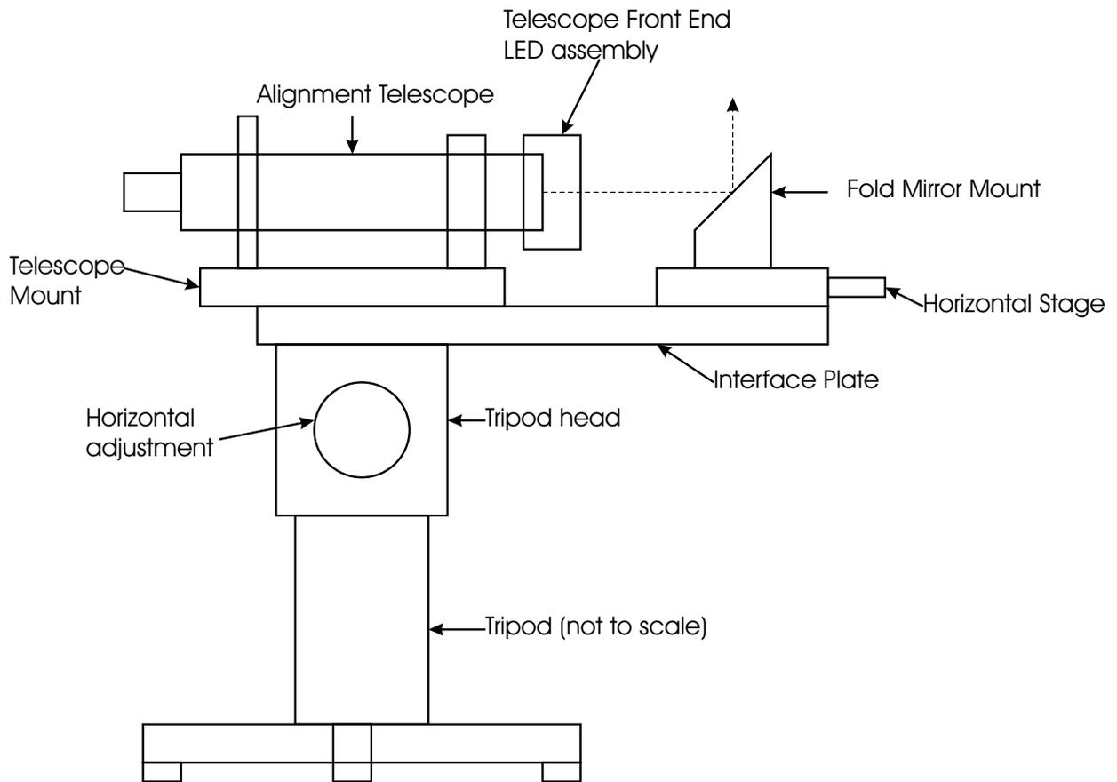
Fig. 1.— Schematic layout (not to scale) of alignment setup, shown for collimator alignment
