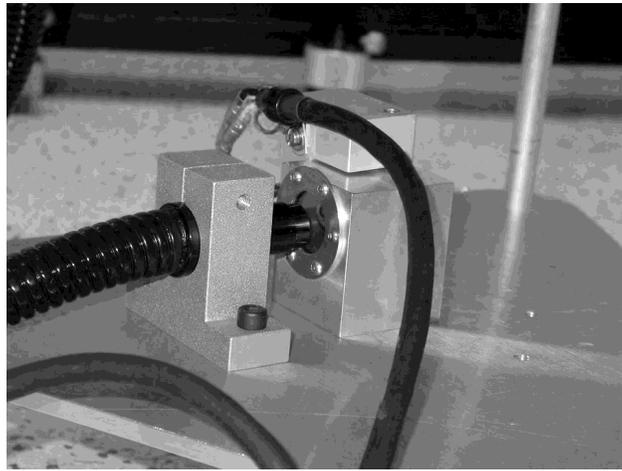
Fig. 5.— QTH lamp block set up for use with the fiber-optic backlight.
