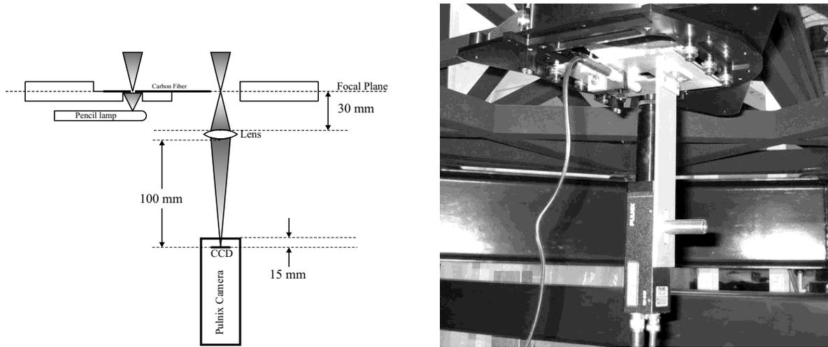
Fig. 3.— Left: Schematic drawing (not to scale) of the autocollimation setup. The pencil lamp illuminates a pinhole cut in a small carbon fiber sheet placed at the center of a modified slitmask holder. The light bounces from the mirror in the collimated beam space returns to the focal plane where the return spot is imaged onto the CCD camera by an intervening lens. Right: Photo of the setup as attached to PFIS.
