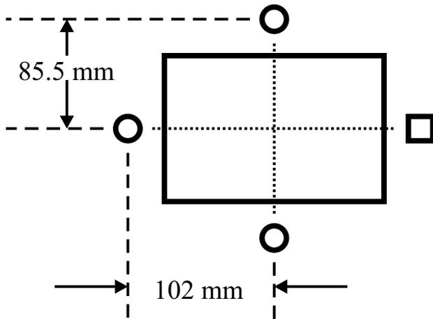
Fig. 2.— Schematic layout for detector interface. There are three screws that allow tip/tilt adjustments. Relevant distances are indicated.
