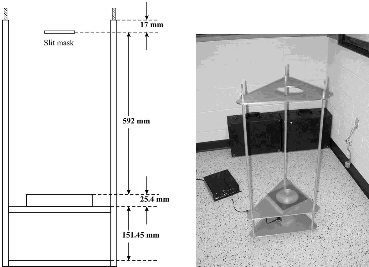
Fig. 4.— Left: Layout of calibration setup with important dimensions labeled. Note: not to scale. Right: Photo of assembled calibration setup with pencil lamp and Fresnel lens. More photos are available at <http://www.sal.wisc.edu/ebb/pfis/pics/assembly/calib/index.html>
